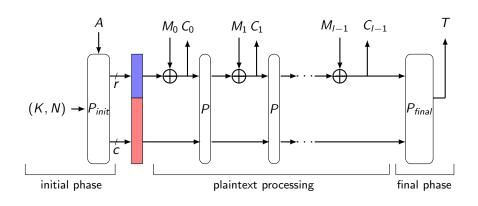
• Permutation P operates on a state of length b = r + c bits, where r is the rate and c the capacity
